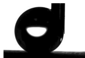
FIGURE 8. Water contact angle of the as-prepared mesh after being dipped in NaCl solution.
